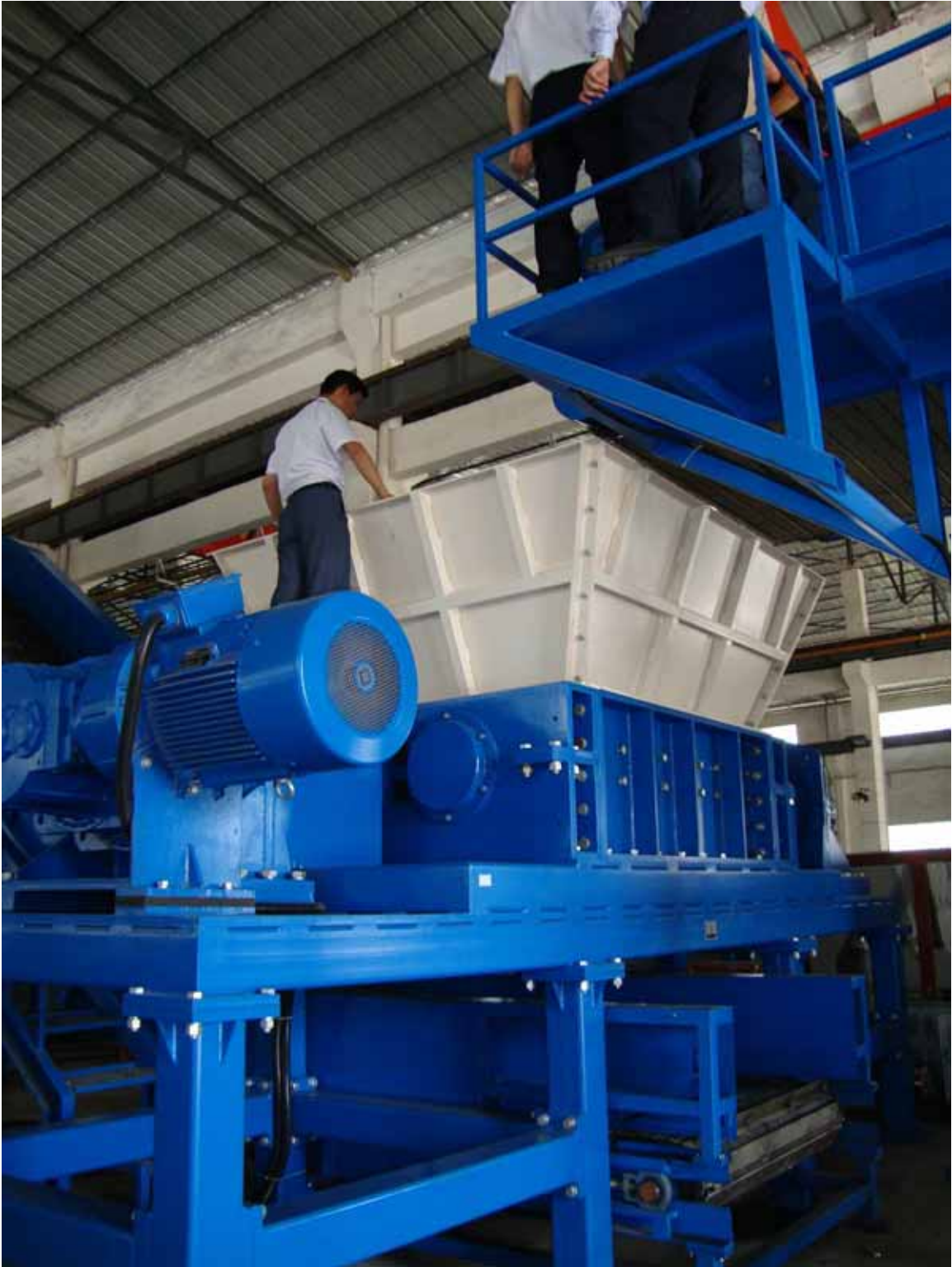
THIS PICTURE ABOVE IS THE SHREDDERHOTLINE.COM EIDAL 7272 UNIT, WITH A 24" SHAFT CENTER DESIGN
