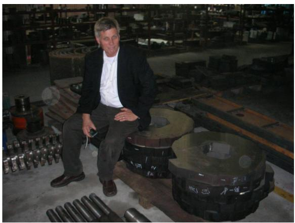
THE PICTURE ABOVE SHOWS THE 34" DIAMTER CUTTER WITH HEX SHAFT DESIGN, THAT YOU WILL FIND IN MANY OF OUR STANDARD PRIMARY SHREDDERS....
