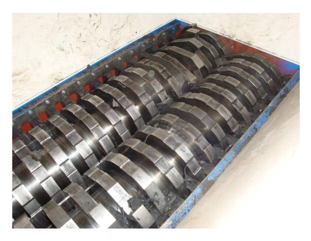
THIS IS A PICTURE OF ONE OF OUR TECHNOLOGIES FOR CUTTERS, THAT ARE USED IN THE PRIMARY AND SECONDARY SHREDDERS, WITH OUR TWO SHAFT MACHINE THAT CUT TIRES, STEEL DRUMS, PALLETS, AND A WIDE ASSORTMENT OF PRODUCTS.....
