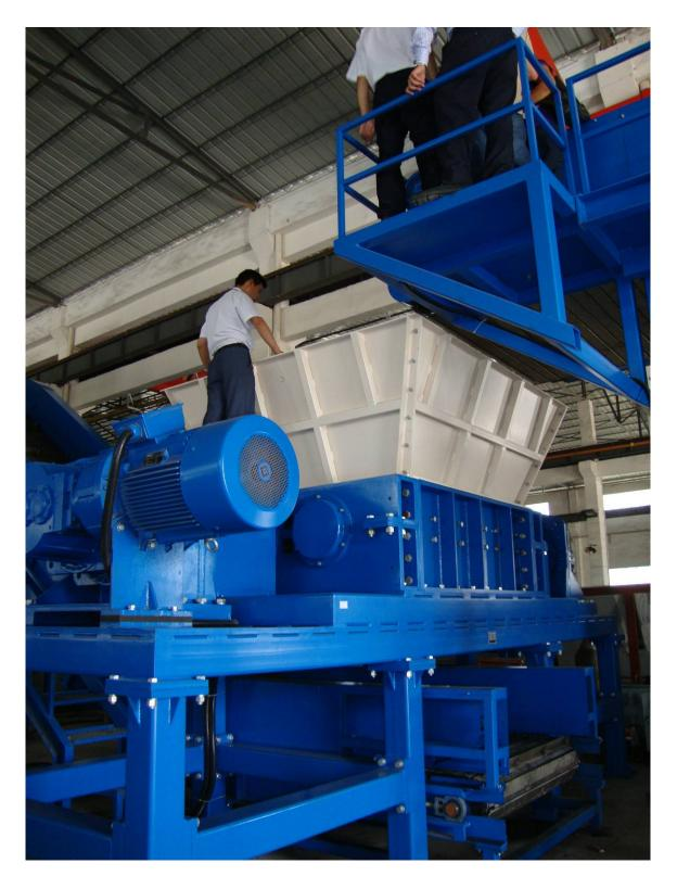
THIS PICTURE ABOVE IS THE SHREDDERHOTLINE.COM EIDAL 7272 UNIT, WITH A 24" SHAFT CENTER DESIGN
