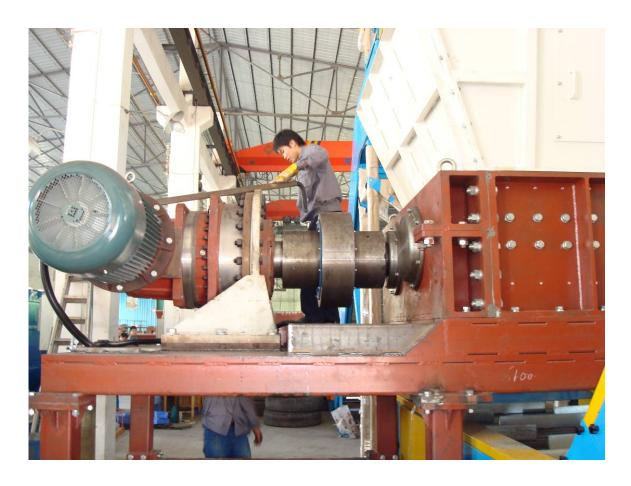
WE ALSO USE A "SPLIT END PLATE DESIGN" WHICH ALLOWS THE CUTTER SHAFTS TO BE REMOVED VERTICALLY AND IN SOME DESIGNS, HORIZONTALLY FROM THE MAIN FRAME OF THE SHREDDER.
