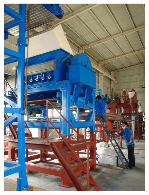
DATA FOR A SECONDARY TIRE RECYCLING SYSTEM TO PRODUCE A WIRE FREE ½″ GRANULE, WITH A DUAL GRANULAR SYSTEM TO MAKE A 10 AND 20 MESH CRUM FROM A
