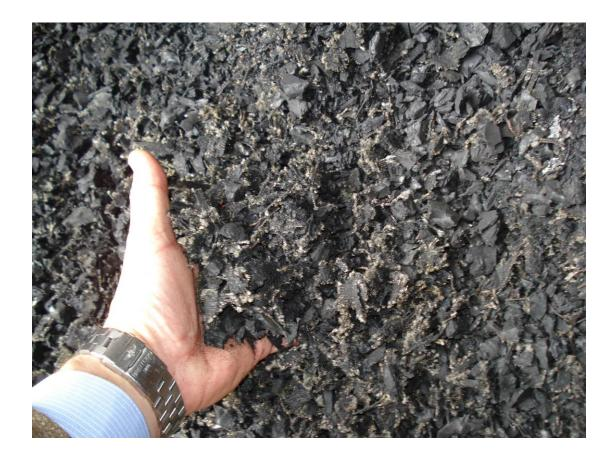
OUTPUT OF GRANULAR PRODUCT FOR THIS SYSTEM IS 4,000KG/HOUR ( 4 TON PER HOUR ) WIRE FREE LANDSCAPE, PLAYGROUND, AND BEDDING MATERIAL, IN THE 6MM ( ¼″ ) AND PREDOMINANT "GRANULAMETRIC CURVE" RANGE OF 12MM ( ½″ ) – GRANULAR TYPE, RECYCLED TIRE MATERIAL
