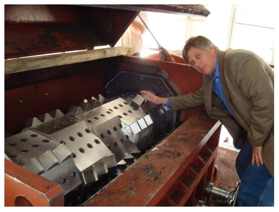
INSIDE VIEW OF OUR 400 HP RASPER DESIGNED TO TAKE TIRE SHREDS TO A ½" WIRE FREE FORM. THE SYSTEM ALSO MAKES CRUM DURING THE PROCESS AND IS SCREENED FROM THE ½" FEED STOCK MATERIAL FOR ADDED PROFIT...
