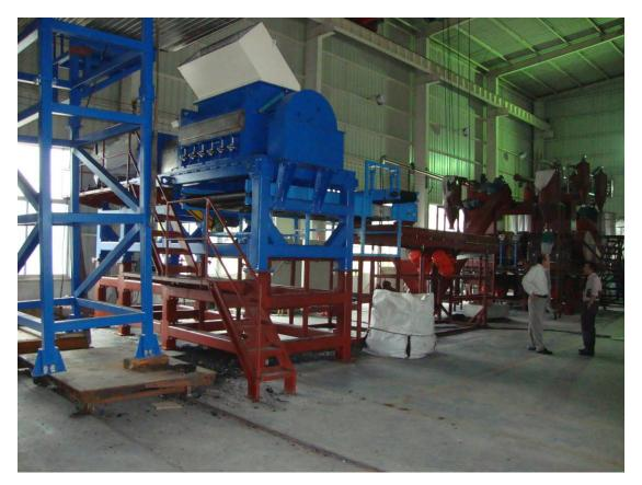
INFEED CONVEYOR AND RASPER TO TAKE PRIMARY SHREDS TO ½" WIRE FREE AND THEN FURTHER TO A 10 AND 20 MESHES
