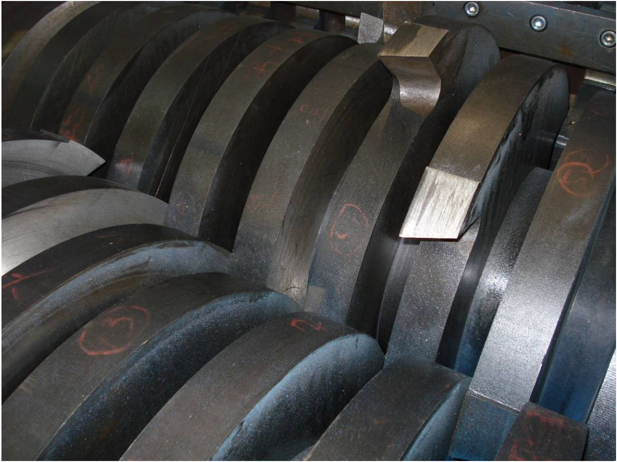
PHOTO ABOVE SHOWS THE EIDAL MODEL 3434 SLOW SPEED SHEAR TYPE SHREDDER CUTTERS ( SERIES 8 ) THAT SHOWS THE CUTTERS THAT GRAB AND CUT MATERIAL INTO STRIP FORM.
