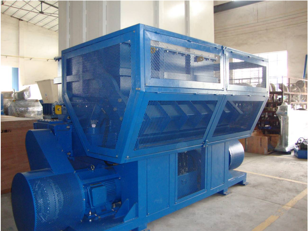
PHOTO OF THE EIDAL MODEL 96-60 SINGLE SHAFT ROTARY GRINDER ( SERIES 1 ) MADE IN 2009 FOR CLIENT IN OHIO
