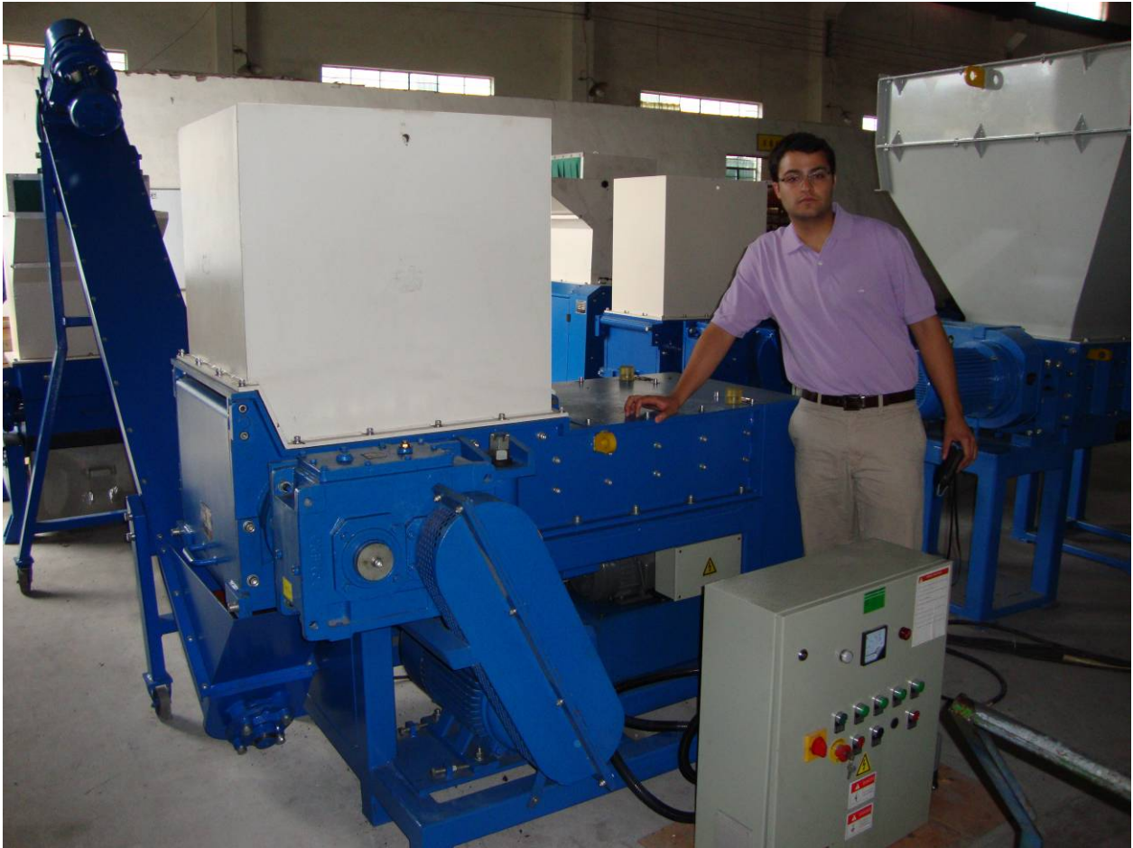
PHOTO OF THE EIDAL MODEL 20-24 SINGLE SHAFT ROTARY GRINDER ( SERIES 4 ) MADE IN 2009 FOR CLIENT IN UTAH
