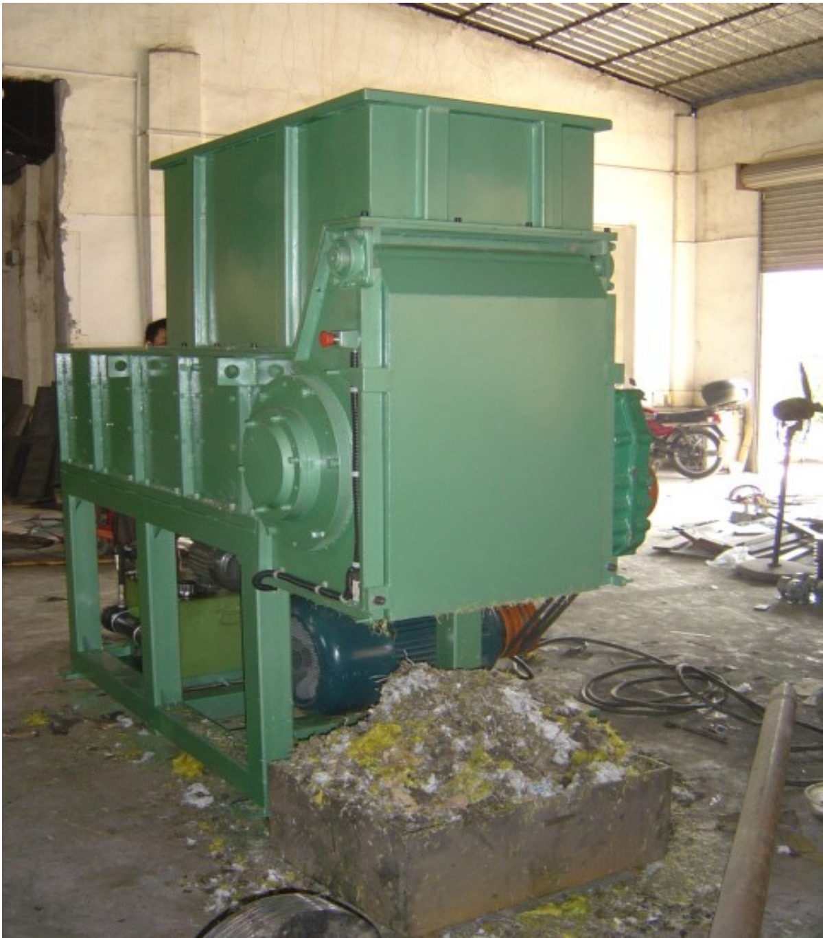
PHOTO ABOVE SHOWS ONE OF THE FIRST EIDAL MODEL 20-24 SINGLE SHAFT ROTARY GRINDER ( SERIES 1 ) MADE IN 1993 FOR CLIENT IN ARIZONA TO PROVIDE CONFIDENTIAL DESTRUCTION OF PLASTIC LABELS
