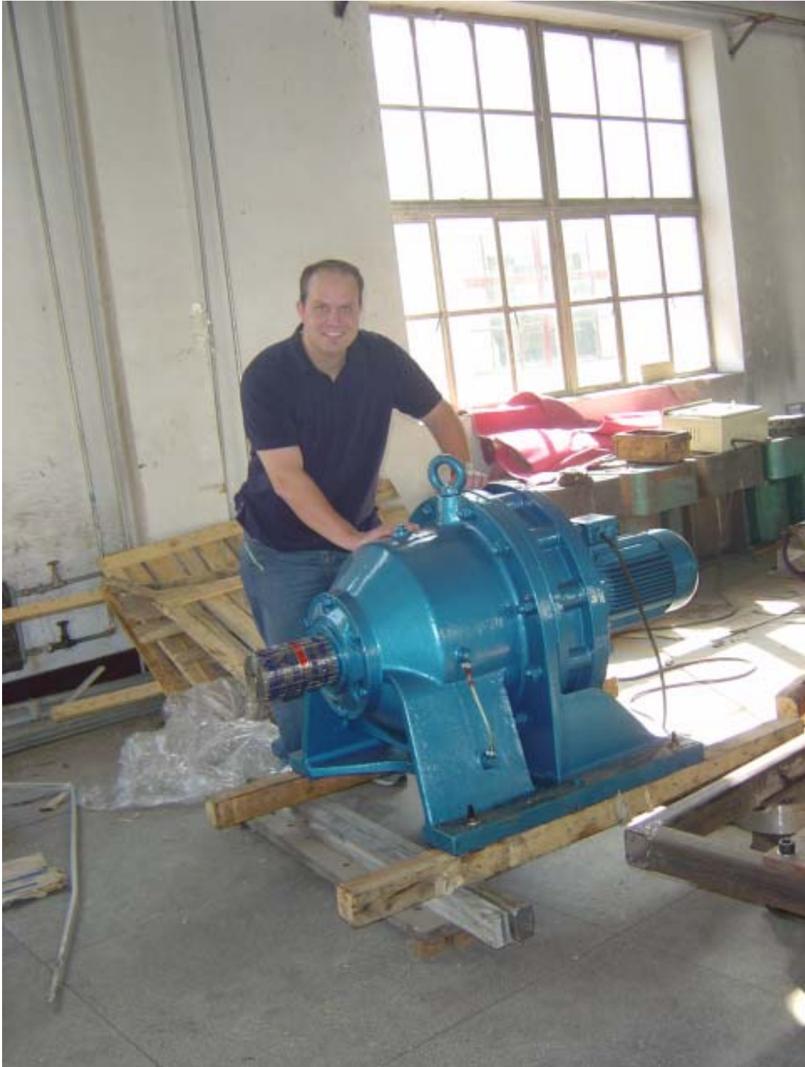
This is one of the two High Ratio Gearboxes that allows us to operate the unit with as low of Hp as 10 HP for many applications.
