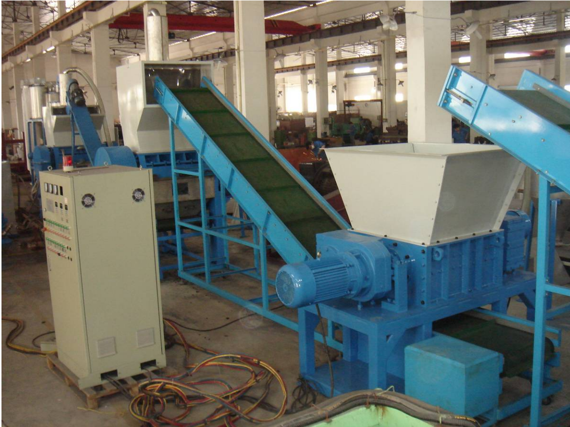
This is a typical linear tire system to make a small granule.
