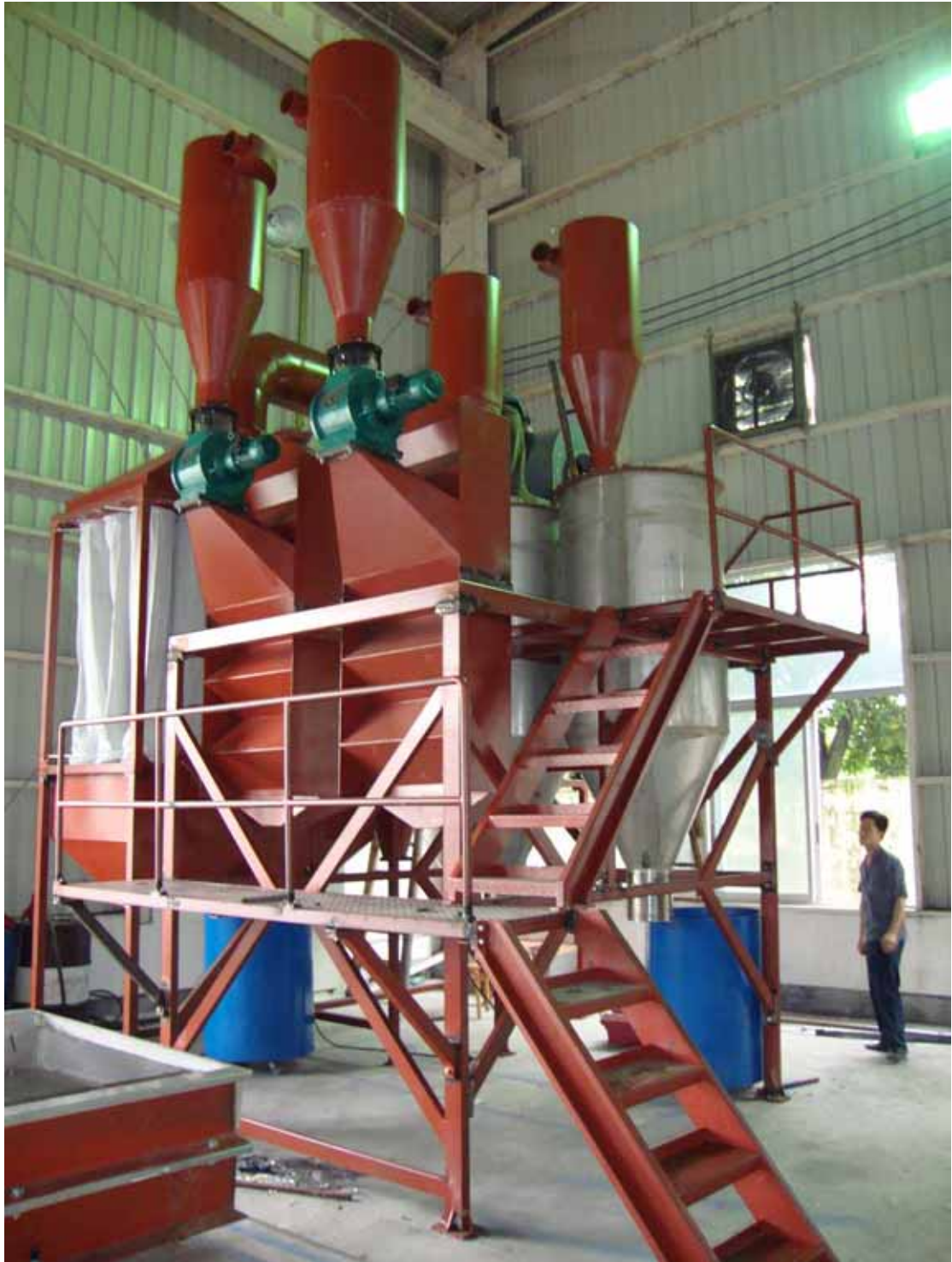
SETUP VIEW OF AIR COLLECTION SYSTEM
