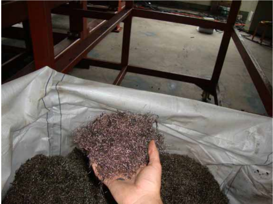
FIRST STAGE VIEW OF WIRE REMOVED FROM TIRE CHIP PRIOR TO SECONDARY CLEANING OF WIRE BEFORE BALING
