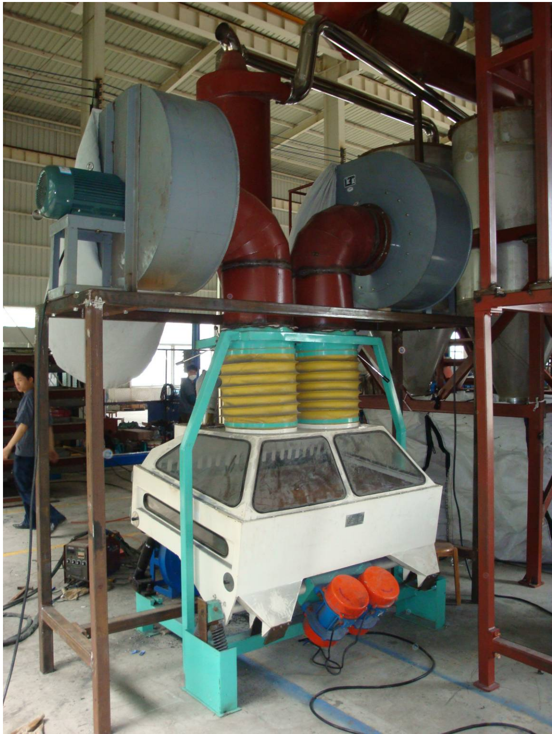
THIS IS THE GRAVITY TABLE WHERE CLEANING OF THE 10 MESH OCCURS
