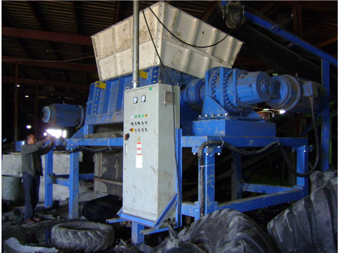
THIS IS A PICTURE OF THE 7272 SHREDDER AT A TIRE PROCESSING FACILITY FOR PROCESSING OTR AND TRUCK TIRES INTO A ROUGH 6" SHRED
